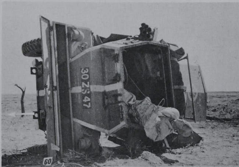
FIGURE 21. ROUND 2. SCOUT CAR AT 1730 ft AFTER FIRING. NO APPARENT DAMAGE TO DUMMY OR SCOUT CAR WHICH SIMPLY TURNED OVER ONTO ITS SIDE
